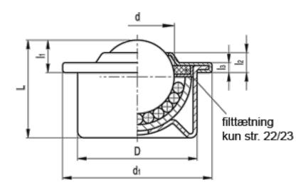
$$\begin{array}{ll} d & = 15.8 \\ D & = 24 \\ d1 & = 31 \\ L + / -0.3 & = 21.0 \\ l1 + / -0.3 & = 9.5 \\ l2 + / -0.3 & = 5 \\ l3 & = 2.5 \\ Max load (N) = 300 \\ \end{array}$$
